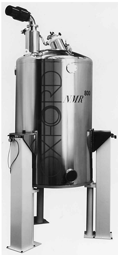
Figure 10. Photograph of a magnet giving the currently highest field (18 T, 800 MHz ^1\text{H} resonance frequency) suitable for magnetic resonance spectroscopy of proteins. Courtesy of Oxford Instruments Ltd.
